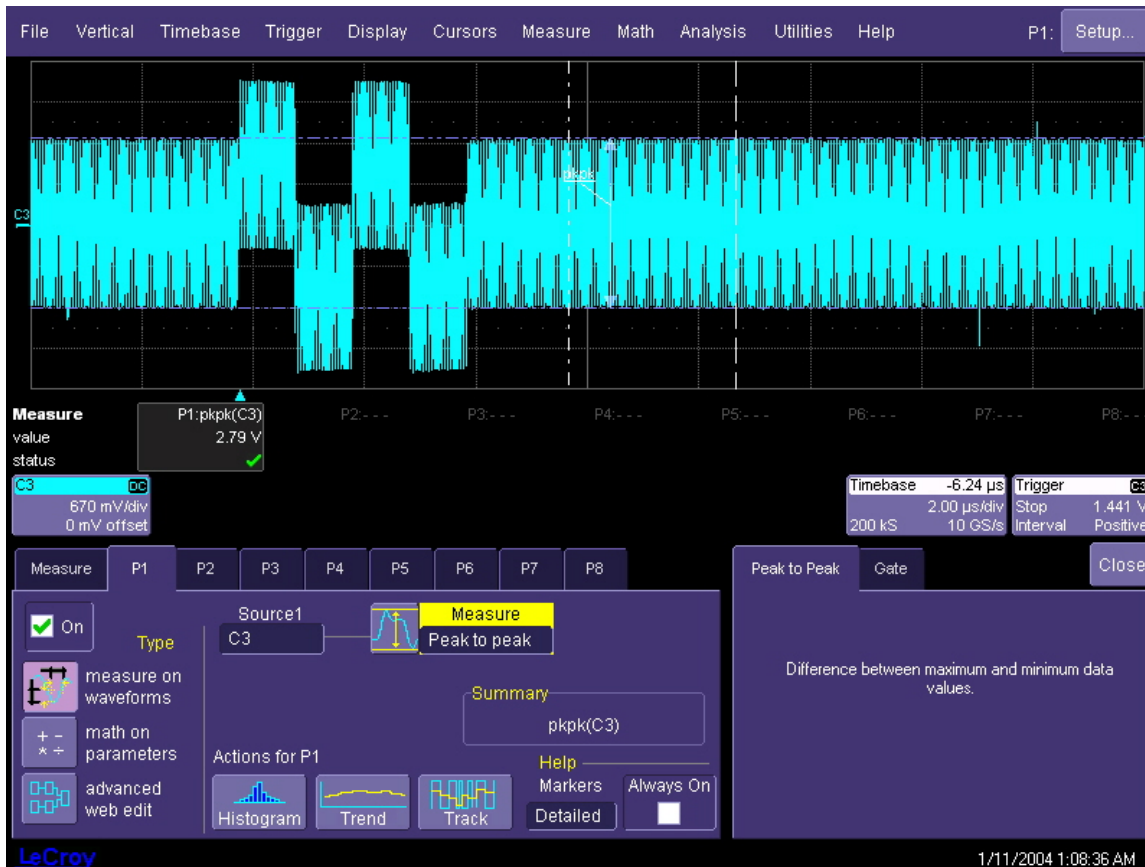
Figure 34: Setting the disturbing signal level for mode 4 test
