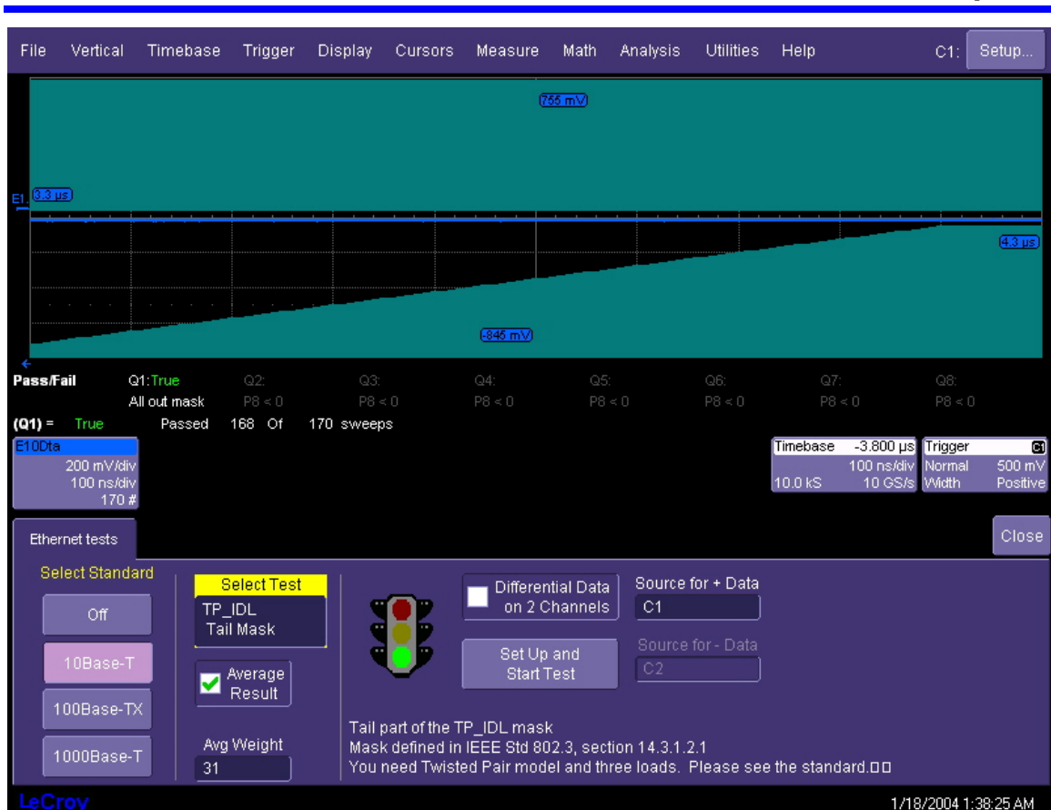
Figure 12: TP_IDL tail mask test
