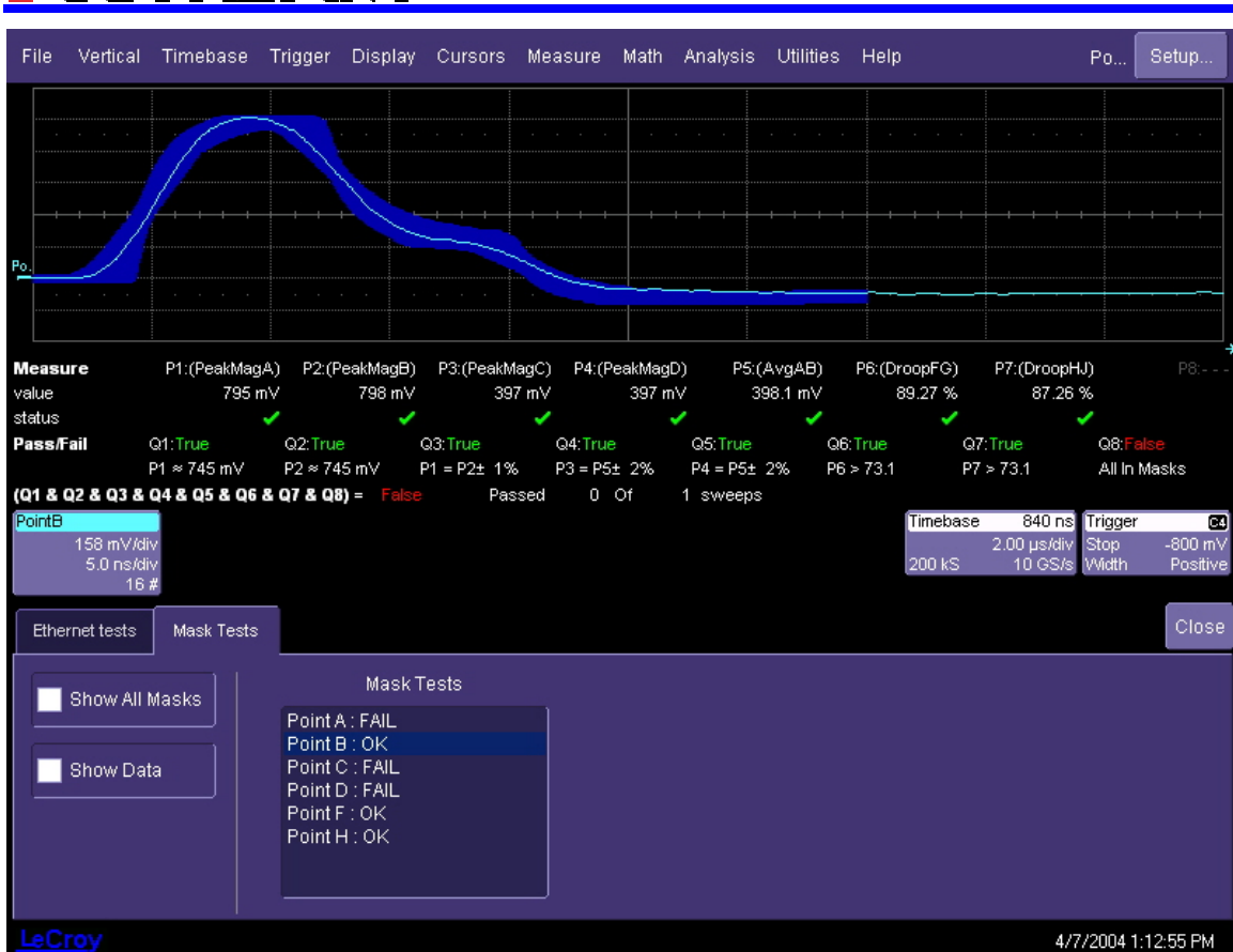
Figure 32: 1000Base-T mode 1 test showing one mask. The mask test results are listed in the menu
