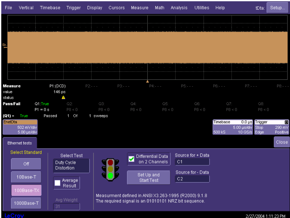
Figure 22: 100Base-TX duty cycle distortion
