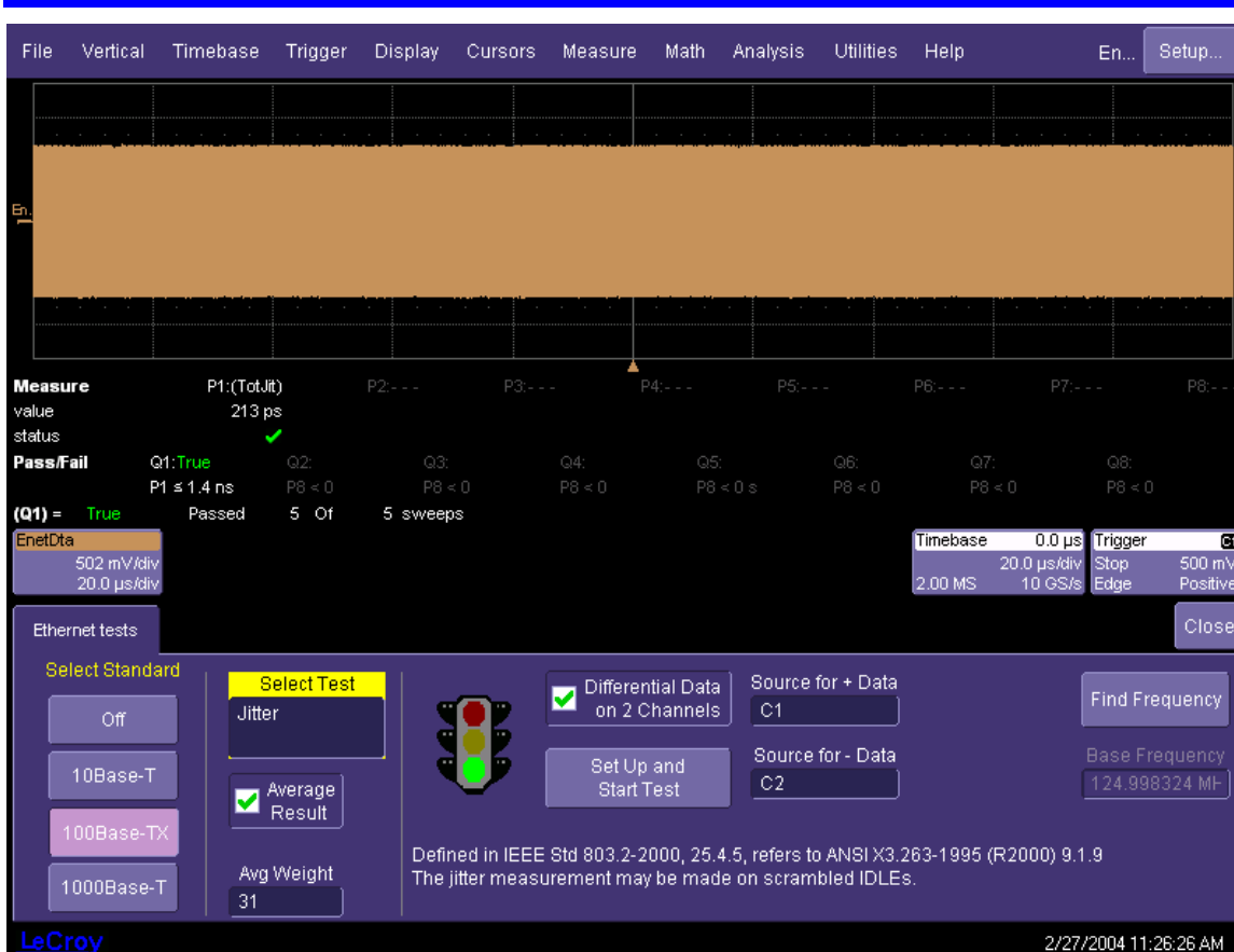
Figure 21: 100Base-TX Jitter Test
